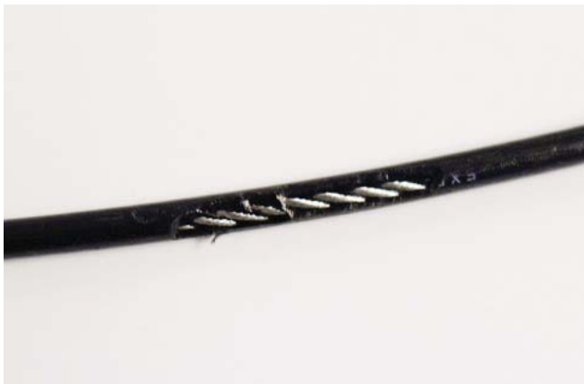
A TEAR IN THE CABLE COVER
