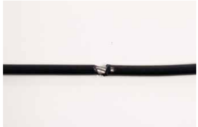
A CRACK IN THE CABLE COVER
