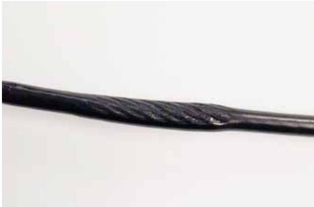
"NECKING", STRETCHED CABLE COVERING
