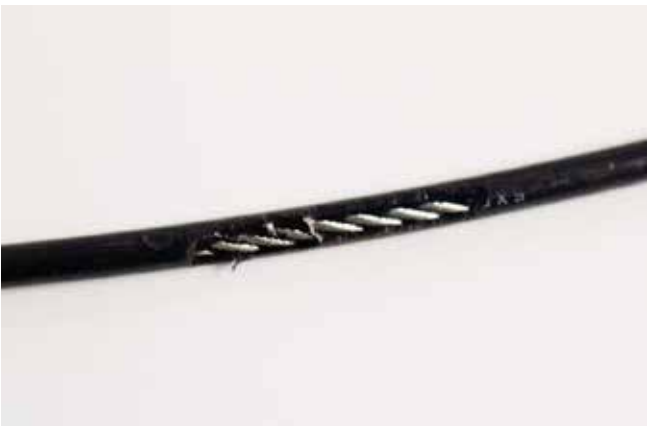
A TEAR IN THE CABLE COVER
