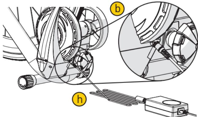
**EN** Insert the resistance unit power cable (h) into the resistance unit (b) as shown. Plug the power supply into the wall outlet. When powered, but not connected to an app or device, the resistance unit status light will blink green.
