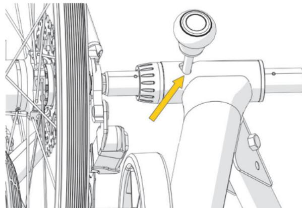
**EN** Pull down the quick release lever to capture the right side of your bike skewer. Quick release handle must be all the way down in locked position.
