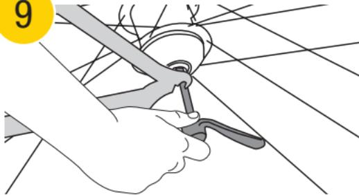
**EN** The trainer is designed to be only used with the provided skewer. Failure to use included skewer may result in damage or injury. Replace the skewer on the rear wheel of your bike with the one provided. Make sure the quick release handle is on the left (non-drive) side of the bicycle and faces upward or backwards.
