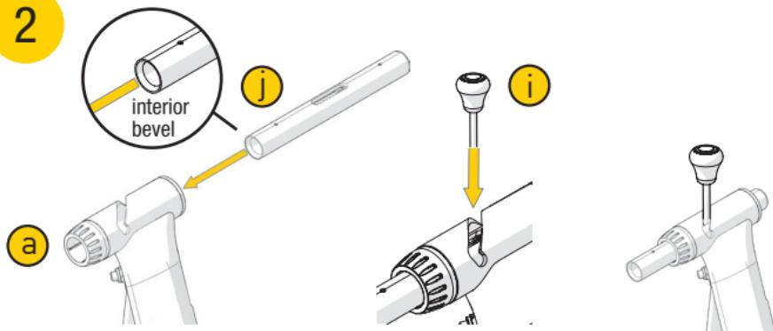
**EN** Insert the bolt action tube (j) into the trainer (a). Insert the quick release lever (i) into the trainer slit and through the center hole of the bolt action tube( j). Tighten the lever (i) into the threads of the bolt action tube (j).
