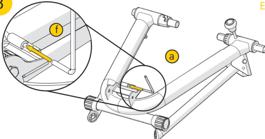
EN Position trainer frame (a) flat on ground with legs folded. Insert L-bolt (f) as shown with arrow.
