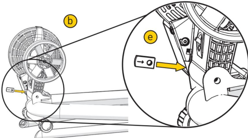
EN While holding the resistance unit (b) in an upright position, insert the nut (e).
