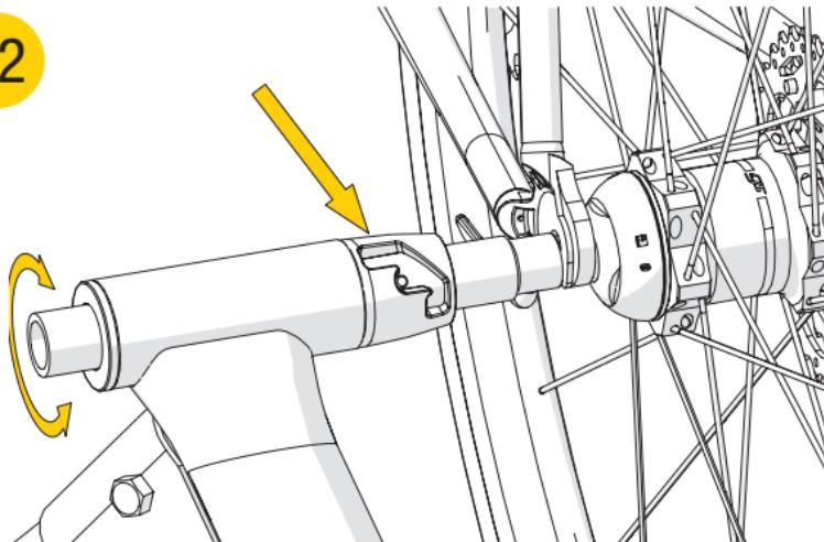
**EN** Adjust the non-drive side of the trainer by pulling the shaft and rotating to appropriate position. Go back to step 11 and engage the quick release handle to secure the bike.
