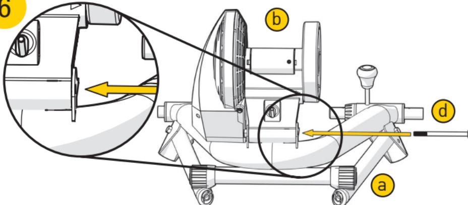
**EN** Guide the bolt (d) into the round hole of the trainer frame (a) as indicated by the arrow. Pass through the resistance unit (b) and secure into the resistance unit nut (e) using a 1/2" wrench.
