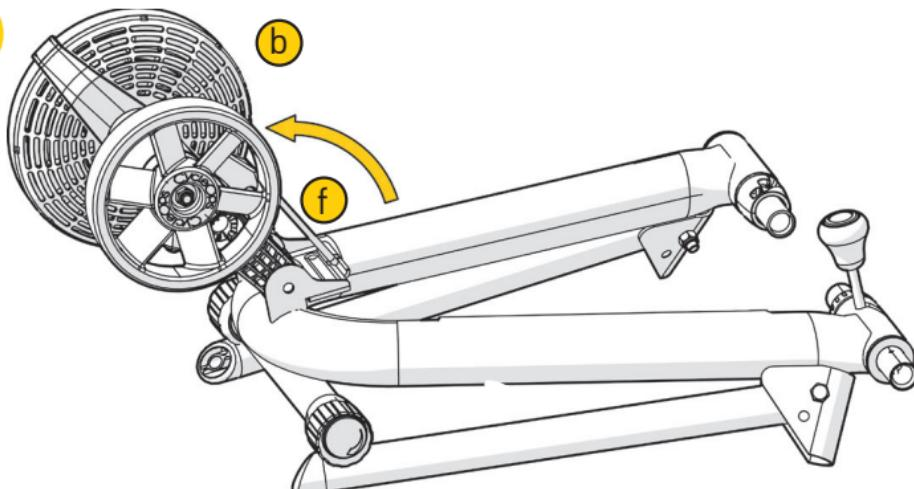
**EN** Place the resistance unit (b) between brackets on the frame and guide the L-bolt (f) through the center of the resistance unit (b).
