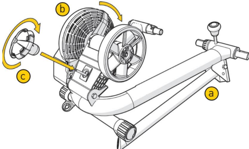
**EN** 1.) Fold the resistance unit (b) into the trainer frame (a).
