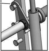
**DANGER:** Pay special attention to the **Weight Lift Bar Assembly (\*20)** making sure both hooks engage uniformly and completely into each **Stopper Prong (#85)**. If both of the Weight Lift Bar Hooks are not engaging uniformly into the **Stopper Prongs (#85)**, it will be necessary to loosen some frame hardware then re-align the frame and re-tighten the hardware. If problem persists, **Do Not Use the Machine** and contact your TuffStuff Retailer or Customer Service (888) 884-8275.
